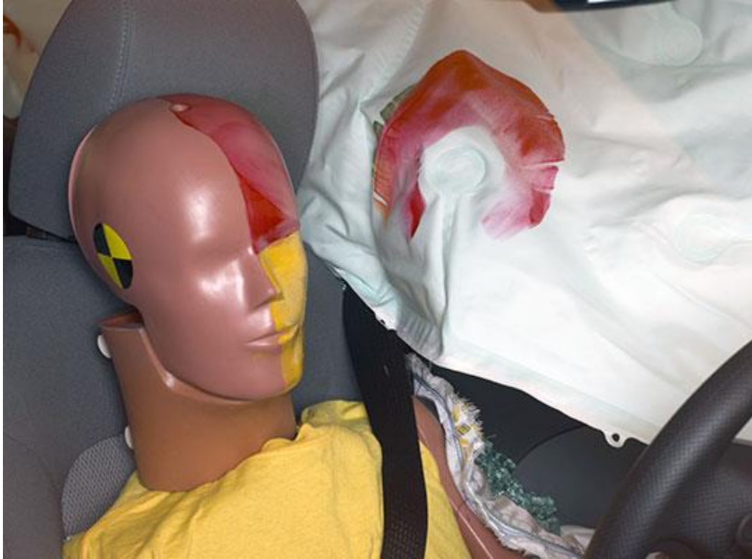
Smeared greasepaint shows where the driver dummy's head hit the side curtain airbag.
